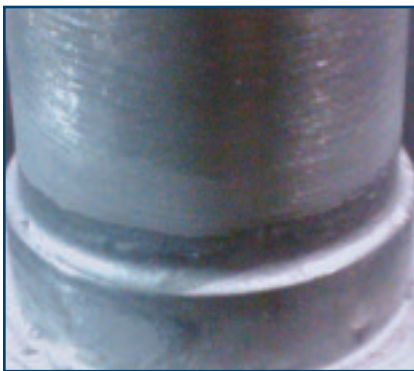
Fig. 3 — Aluminum tube-to-fitting joint using induction heating and AWS A5.8 BAlSi-4 filler metal.
