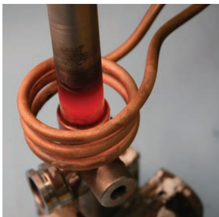
Examples of various assemblies heated to brazing temperature using induction heating.
