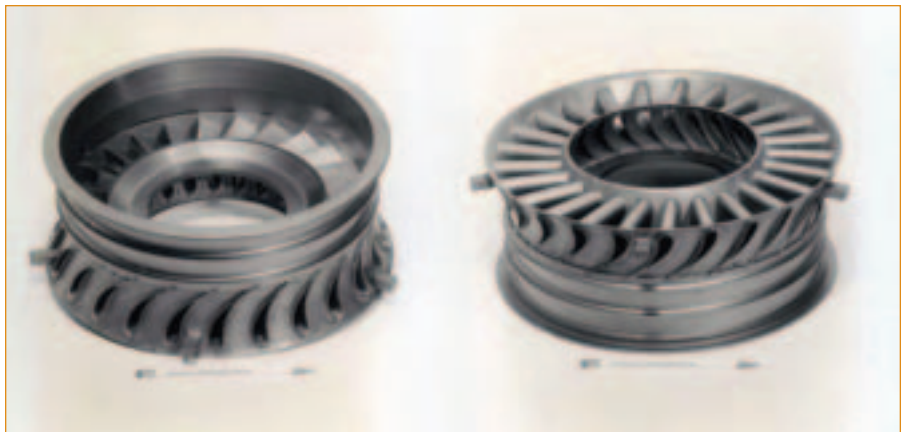
Fig. 4 — Because fitup for the joint edges on these gas engine turbines was not well controlled, a sluggish filler metal such as BNi-1 was needed.
