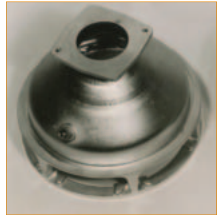
Fig. 3 — The interior of this part, the housing for a jet engine starter, experiences high temperatures and high stresses and the joint has tight fitup, which necessitates the use of a free-flowing alloy such as BNi-2 or BNi-3.
