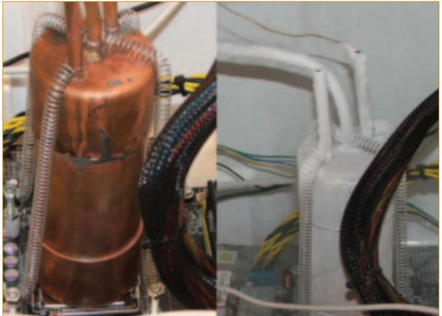
Fig. 3 — Computer installed within automated refrigeration system, wherein liquid N<sub>2</sub> is the working fluid. The Cu evaporator is pictured (Ref. 12).
