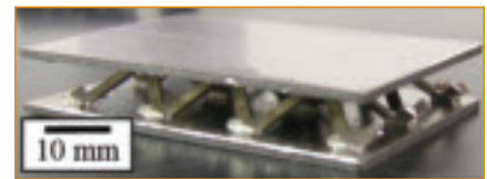
Fig. 1 — Examples of the geometry of titanium pyramidal core with and without brazed facesheets.
