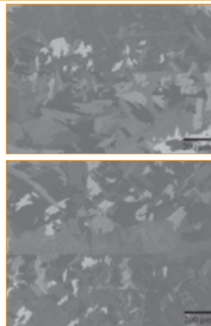
Fig. 4 — High-magnification images of a Ti-6Al-4V interface resulting from DB+HIP (top) and Braze+HIP (bottom).
