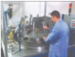
Rotary Index Machine 400 parts per hour
