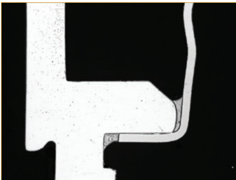
Complex lap joint made with Sn-Sb solder for a high-reliability assembly.
