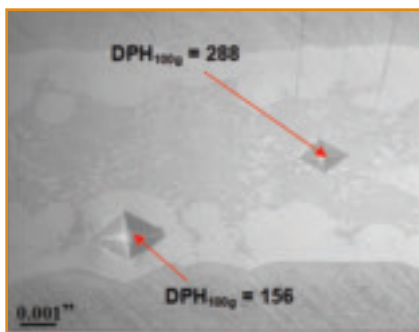
Fig. 19 — Alloy 152 section from horizontal variable clearance test showing microhardness indents within a brazed joint of approximately 0.006 in. ( \sim 0.15 mm).
