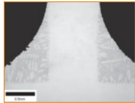
Fig. 13 — Metallographic cross section of a brazed Alloy 31 T-piece.
