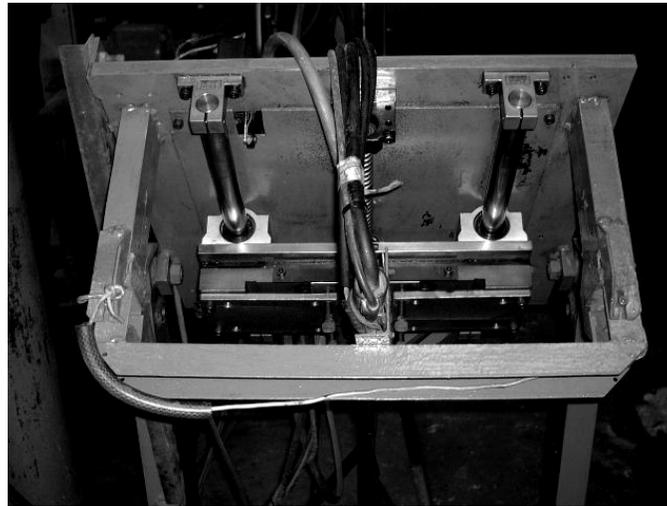
**Figure 1. Welding table designed for the 10-h position welding experiment**
