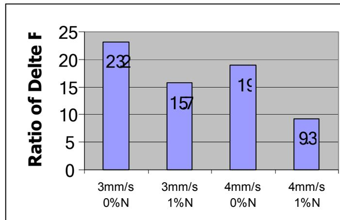
Figure 6. The ratio of delta ferrite in austenite matrix of specimens welded by using pure Ar gas and Ar gas mixed with 1 vol.% of nitrogen at the welding speed of 3 and 4 mm/s. (Welding condition: pulse frequency of 7 Hz, 45% on time, base current of 43 A.)
