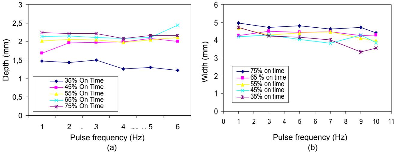
**Figure 2. Depth(a) and width(b) of weld metal as a function of pulse frequency at different percents on time. (Welding condition: base current of 43 A, pulse current of 105 A and welding speed of 3 mm/s)**
