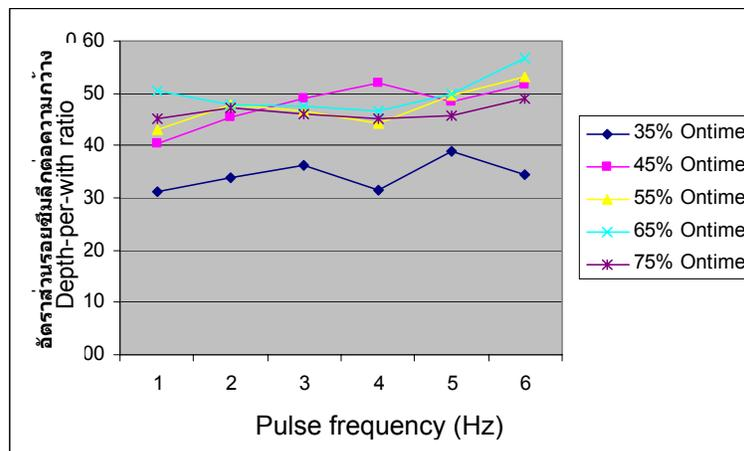
**Figure 3. Depth-per-width ratio of weld metal as a function of pulse frequency at different percents on time. (Welding condition: base current of 43 A, pulse current of 105 A and welding speed of 3 mm/s)**
