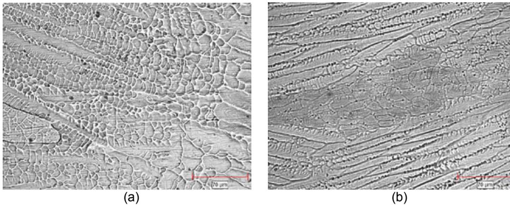
Figure 5. Microstructure of weld metals of specimens welded by using (a) Ar shielding gas, (b) Ar shielding gas mixed with 1 vol.% of nitrogen gas. (Welding condition: pulse frequency of 7 Hz, 45% on time, base current of 43 A, pulse current of 155A and the welding speed of 4 mm/s)
