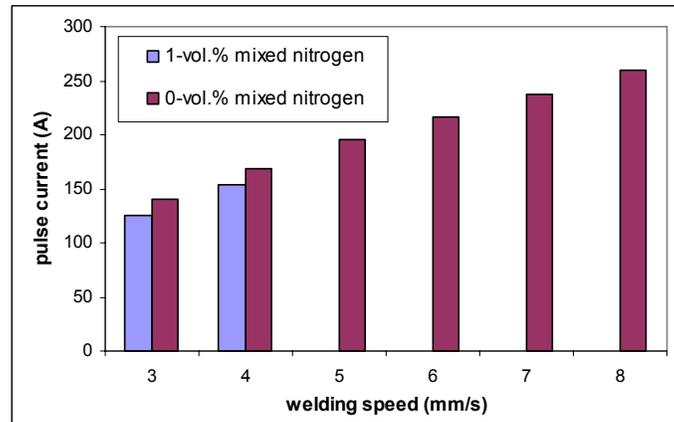
Figure 4. The pulse current that gives rise to the weld bead shape correspond to DIN 8563 quality class BS ( $I_p^*$ ). (Welding condition: pulse frequency of 7 Hz, 45% on time and base current of 43 A)
