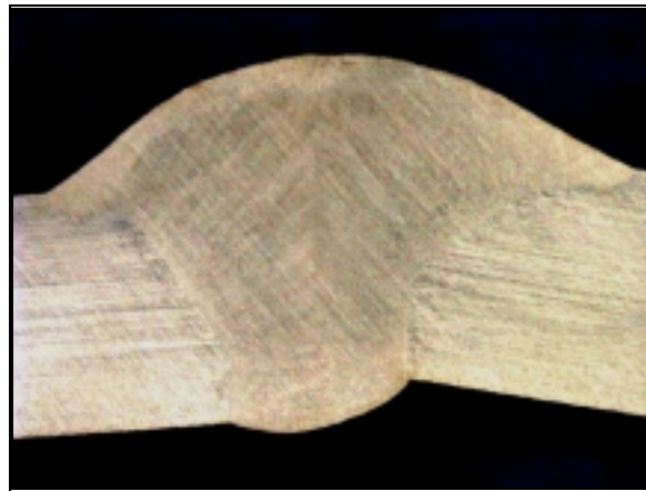
Macrograph showing poor fit-up (butt weld)
