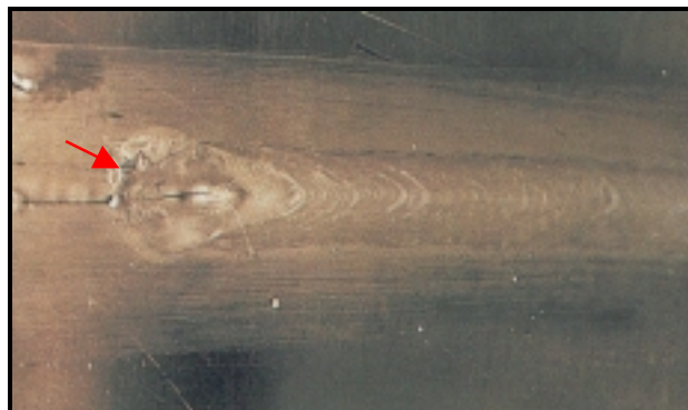
Photograph illustrating crater cracking resulting from abrupt weld termination in an aluminum weld (MIG process)
