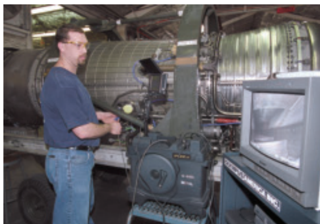
Fig. 2 — An inspector at Tinker Air Force base gets a magnified view of an engine's high-pressure turbine area with a new digital fiber-optic borescope. (Photo courtesy of U.S. Air Force; photo taken by Margo Wright.)
