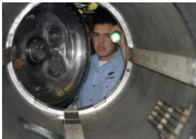
Fig. 1 — Visual inspection of a torpedo tube aboard a Navy attack submarine. (Photo courtesy of the Department of Defense; photo taken by JO3 Corwin Colbert, USN.)
