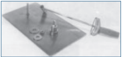
Fig. 3 — Method of applying a tensile load to a welded stud using torque. A bolt can be used for an internal thread.
