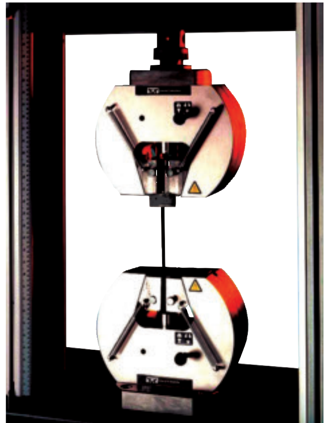
Fig. 1 — Shown are Instron® 100-kN pneumatic wedge-action grips, which help to maintain accurate alignment of the specimen during tensile testing. (All photos courtesy of Instron®.)
