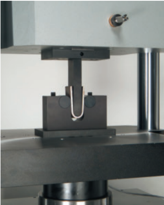
Fig. 2 — A guided bend test on a welded sample.
