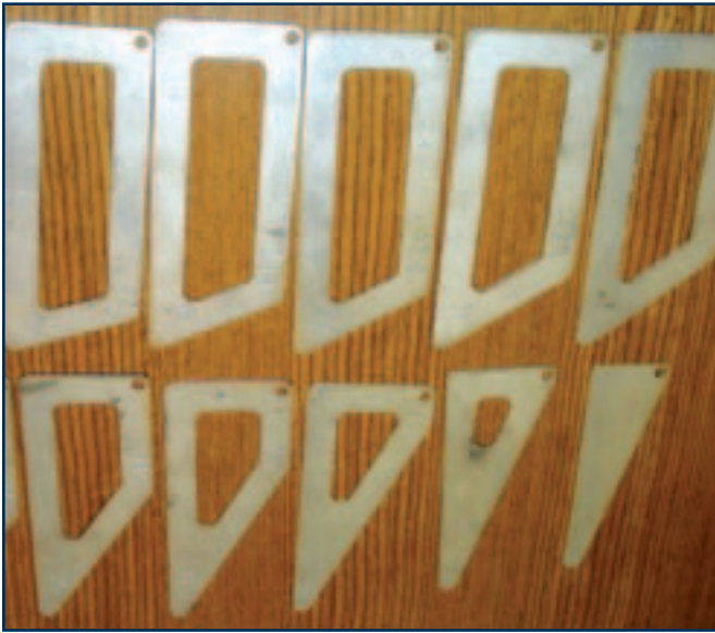
Fig. 5 — A few of the dihedral angle gauges Mankenberg often uses in his work.
