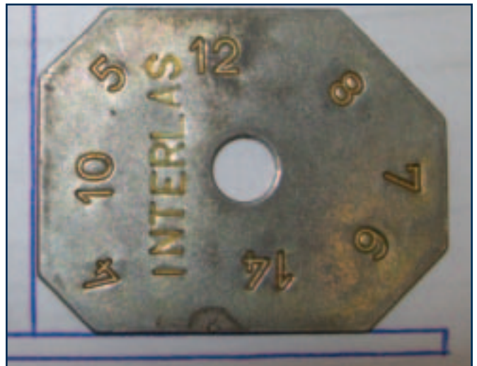
Fig. 2 — A simple one-piece fillet weld gauge can solve a lot of problems.
