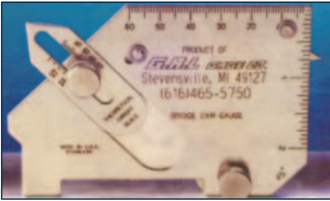
Fig. 3 — The bridge cam gauge can be a multipurpose godsend for professional inspectors.
