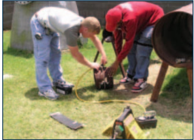
Fig. 3 — Two students carefully set up an X-ray system for evaluating welds made on a section of pipe.
