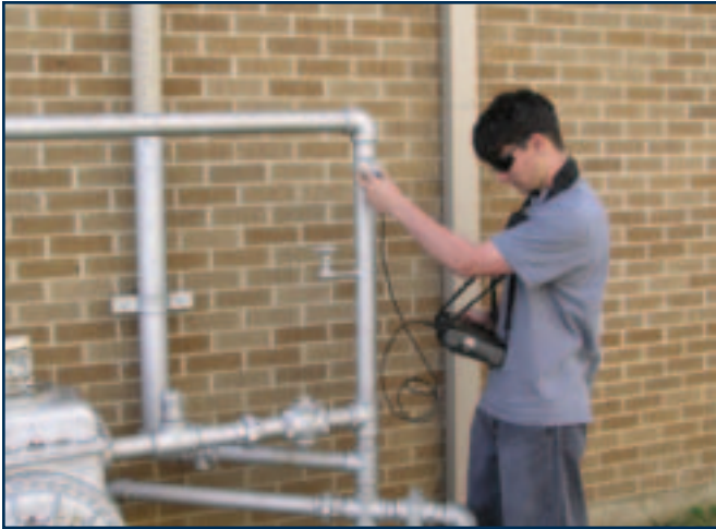
Fig. 2 — A student uses his acquired skills to perform ultrasonic testing on small-diameter pipes.
