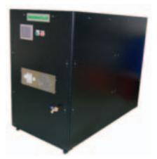
The MagnaPure II® uses ozone to remove the green dye color from fluorescent penetrant rinse water. The unit can process up to 500 gal of rinse water per 24-h period. It eliminates the use of filters and/or cartridges. It requires minimal floor space and maintenance, reduces bacteria and odor problems, and features a separate sample valve, an easy-to-use color touch screen, and drop-in installation. No penetrant residue or sludge is left after the filtration process.
