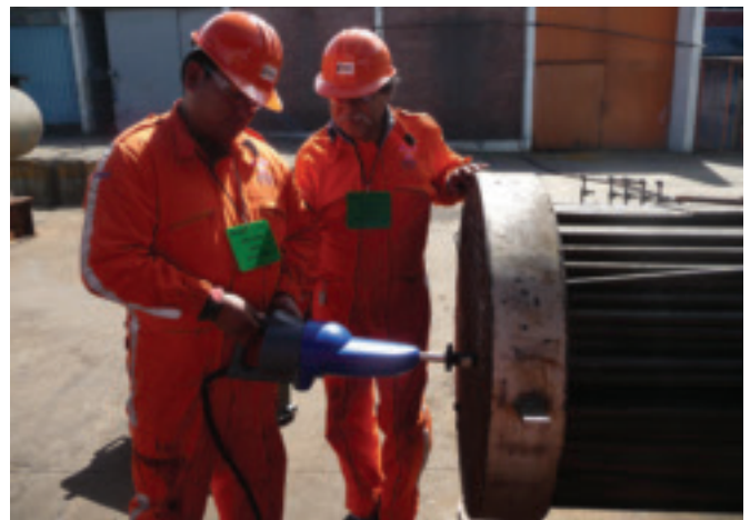
Fig. 2 — The acoustic pulse reflectometry system in use. It can detect such discontinuities as holes, pits, wall loss, and bulges.
