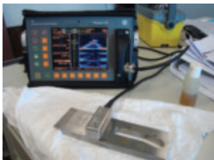
Fig. 1 — The latest phased array equipment, such as the Phasor CV/DM from GE Sensing & Inspection Technologies, uses multiple ultrasonic elements and electronic time delays. Advantages include repeatability, speed of inspection, and capability for inspecting complex geometries. Shown is the screen shot of the reference block.
