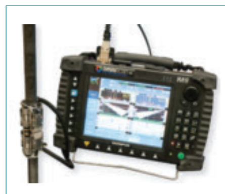
Fig. 2 — Two-sided scan being performed on small-diameter vertical pipe.
