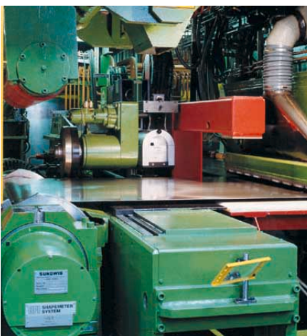
Thickness and flatness measurement on the 20-roll cold rolling mill.
