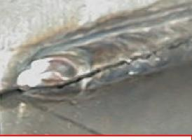
Crack caused from unfilled crater
