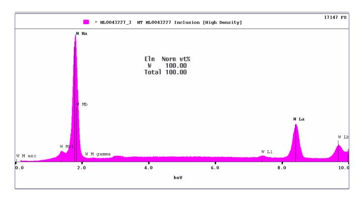
**Note:** SEM/EDS analysis is semi-quantitative method of detecting elements with an atomic number of five (Boron (B)) or greater that are present in minimum quantities of approximately 0.1%. The relative percentages of the elements detected are quantified and normalized to 100%. Therefore, these results must be treated as relative, not absolute, quantities.
