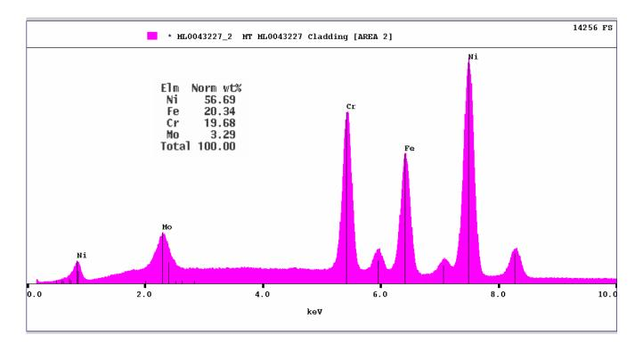
Note: SEM/EDS analysis is semi-quantitative method of detecting elements with an atomic number of five (Boron (B)) or greater that are present in minimum quantities of approximately 0.1%. The relative percentages of the elements detected are quantified and normalized to 100%. Therefore, these results must be treated as relative, not absolute, quantities. MATFORM.004
