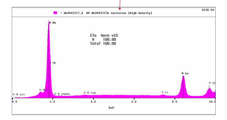
Note: SEM/EDS analysis is semi-quantitative method of detecting elements with an atomic number of five (Boron (B)) or greater that are present in minimum quantities of approximately 0.1%. The relative percentages of the elements detected are quantified and normalized to 100%. Therefore, these results must be treated as relative, not absolute, quantities. MATFORM.004
