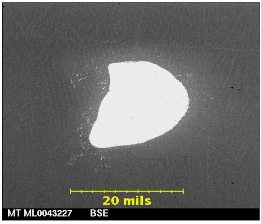
**Note:** SEM/EDS analysis is semi-quantitative method of detecting elements with an atomic number of five (Boron (B)) or greater that are present in minimum quantities of approximately 0.1%. The relative percentages of the elements detected are quantified and normalized to 100%. Therefore, these results must be treated as relative, not absolute, quantities.
