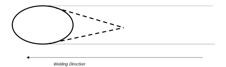
Solid Line = Low Welding Speed Pool Shape
