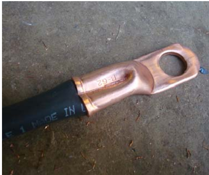
Figure 2.3: Copper lug on work lead / cable.
