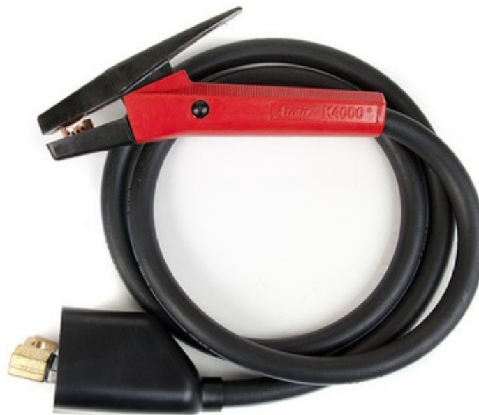
Fig. 2.1 Arc Air: K4000, notice the model number on the handle.
