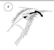
5. Stay in the puddle and move the electrode back across the gap. Move the electrode down the joint in a half-moon motion.
