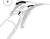
9. End the weld at 6 o'clock by moving the arc onto the sidewall.
