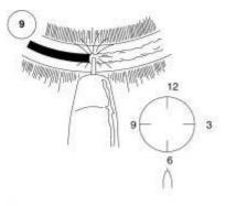
10. DO NOT stop welding while in the root. This may cause pin holes.
