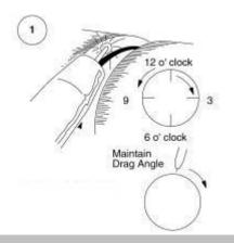
2. After puddle is established, maintain the arc on the forward portion of the puddle.
