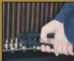
Hand tool lifts tube from seal.
