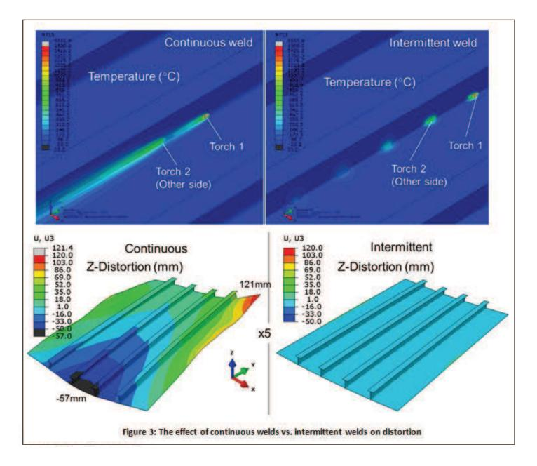
concepts to predict which method or combination of methods will be most effective. As an example, numerical models have been developed to determine pre-cambering shape and magnitude for distortion control. Figure 3 illustrates the use of numerical modelling to evaluate intermittent welding as a method of eliminating buckling distortion.
