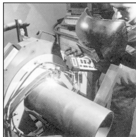
Fig 1. Orbital TIG welding of tube.
