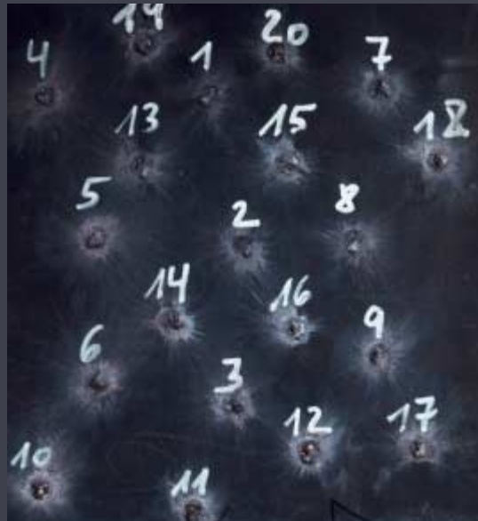
Cover/rear photo: Ultrafort specimen after testing with hard-core ammunition
