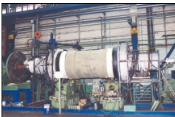
Figure 3: Overlay Weld in the Shaft Seal Area for a Nuclear Power Plant
