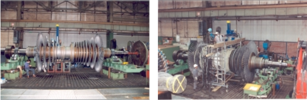
Figure 7: Build-up Weld Repair of Creep Damaged Stage
