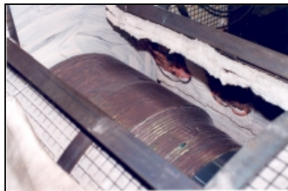
Figure 3: Overlay Weld in the Shaft Seal Area for a Nuclear Power Plant
