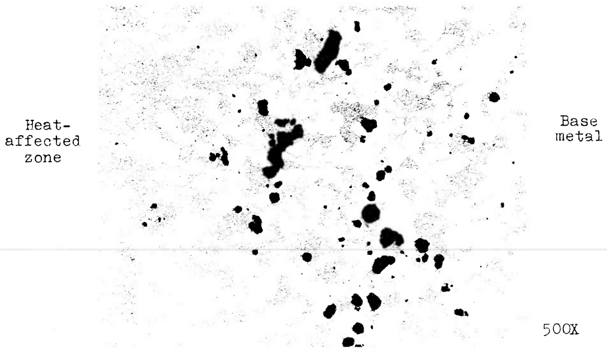
Fig. 2. Photomicrograph of the graphitized zone in the cracked valve material shown in Fig. 1.
