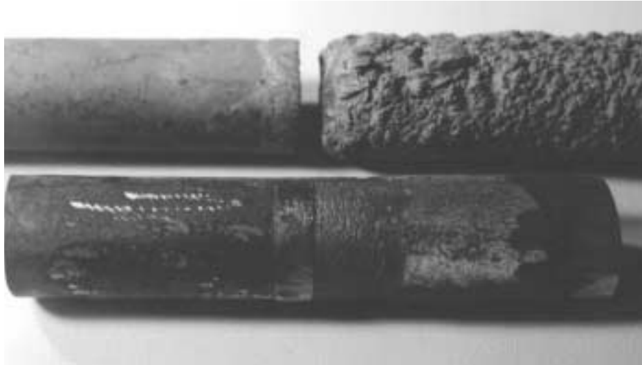
Figure 3 Macrograph of DMW Samples The top tube exhibits features typical of a DMW failure. The failure of this tube prompted examination of the bottom tube, Sample D.
