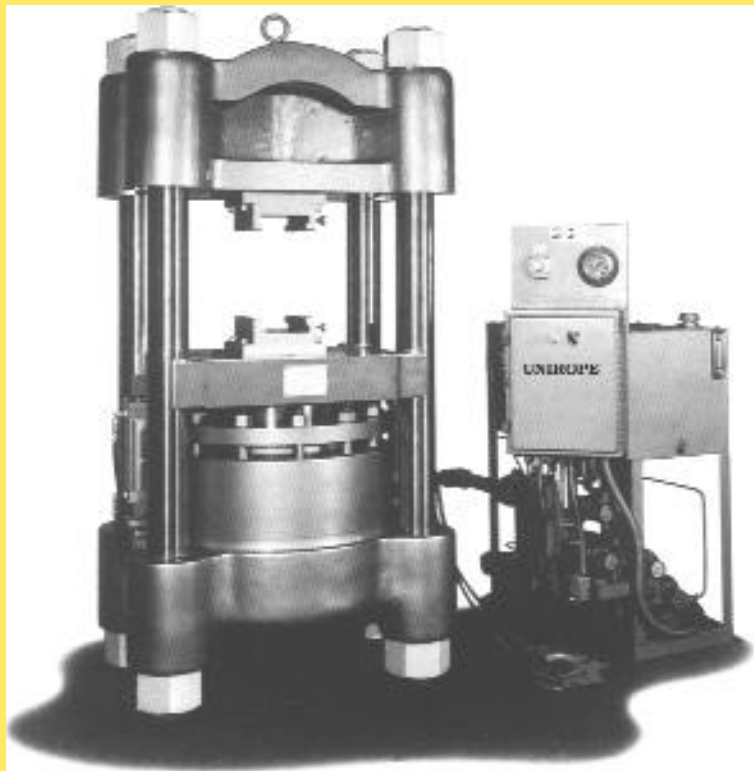
1500 ton swager for wire rope flemish eye slings up to 2-1/2" diameter. One of a total of 8 rope swagers to meet any and every demand.
