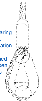
Check sling for broken wires. Flexing the rope exposes hidden wire breaks.
