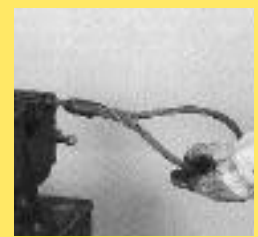
The ends of the strands are laid around the body. The eye is ready and develops about 70% of the required sling strength.
