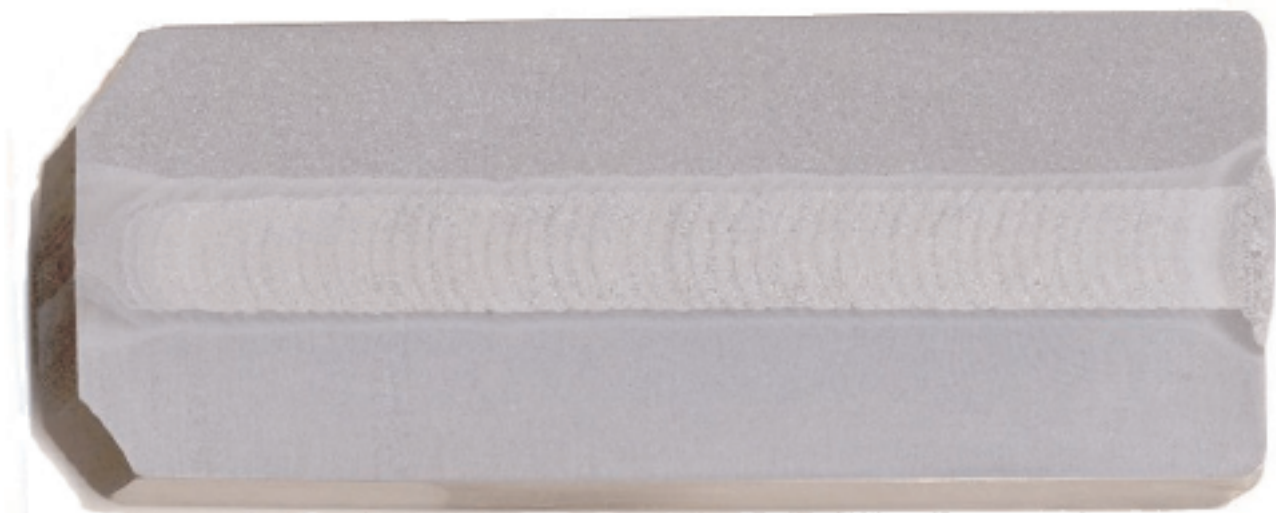
Figure 3 Macrosection through full-scale weld
