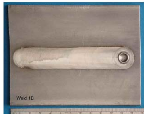
Figure 8. Friction stir processing trial - stainless steel
