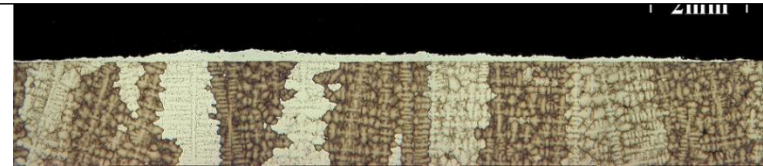
Coating microstructure and associated variation in thickness taken using quantitative microscopy
