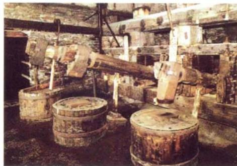
Figure 8.1.10: Water-powered hammer-forge at Bentsberg, Germany
