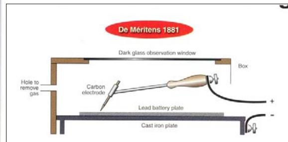
The process was carried out in a box with a fixed electrode.
