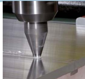
**friction stir seam weld**
