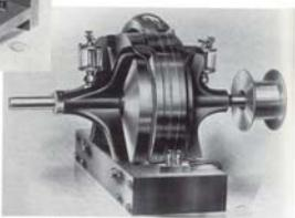
Figure 3.2.2: First Tesla AC motor
