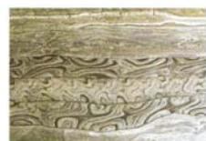
Figure 8.1.3: Patterned steel created by forging
