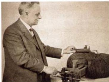
Figure 7.4: Elihu Thomson with first electric welding transformer with a single-turn secondary built in early 1886
