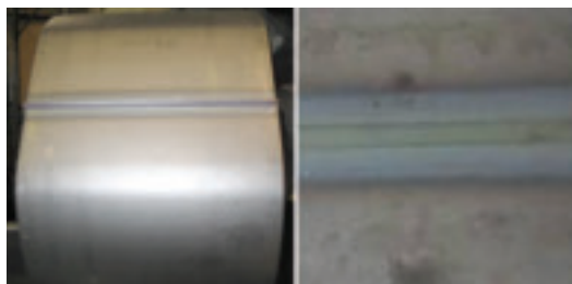
Fig. 4 — Rim manufacturing process, weld joint with fin surface after scarfing process.
