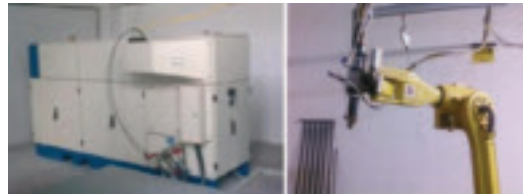
Fig. 6 — Nd:YAG 4000-W laser machine and robot welding mechanism.
