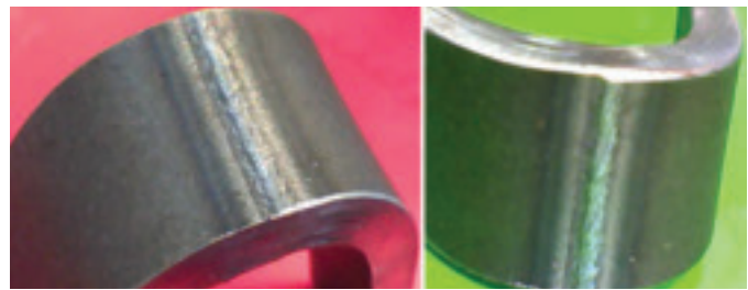
↑ Fig. 13 — Laser welded specimens to which bending tests were applied.
