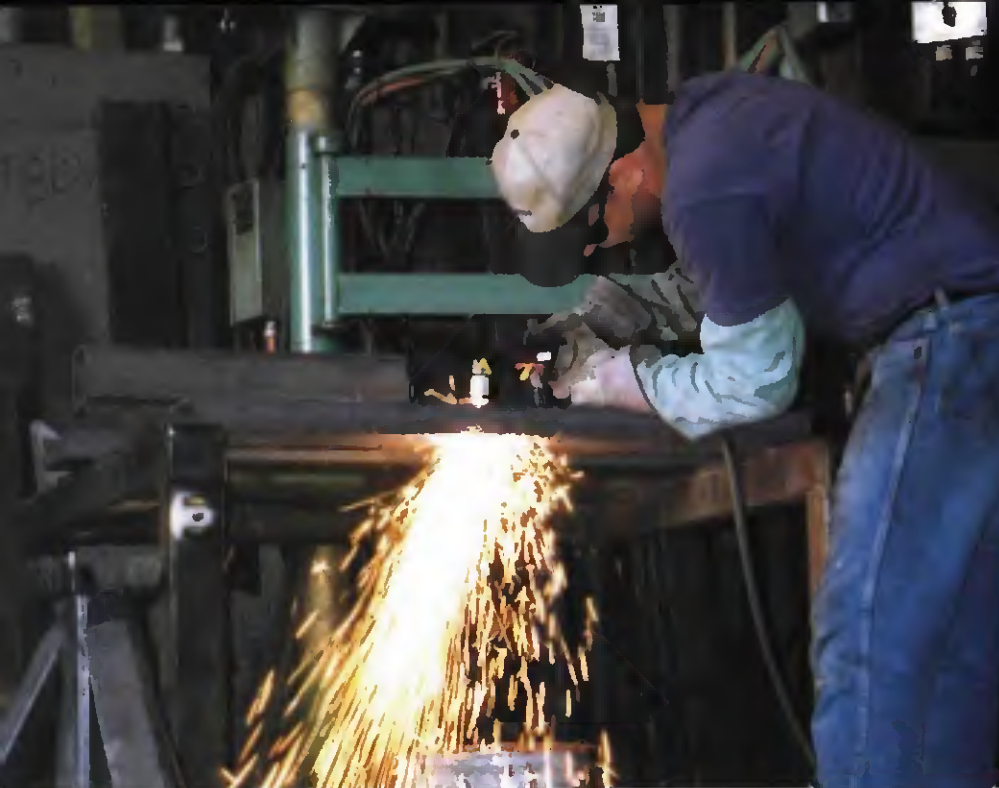
Fig. 1 — Dave Robertson of Peterson Manufacturing cuts caps out of 1/4-in. mild steel.
