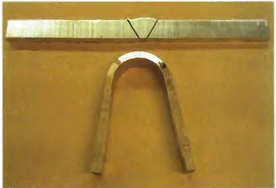
Fig. 1 — Guided bend test samples. Top sample shows a side bend section prior to full preparation and bending. Lower sample shows a completed side bend specimen.
