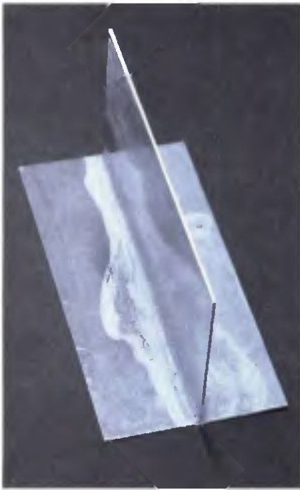
Compos of Alloy 6111 soldered using Zn/15Al and a flux based on complex fluoroaluminate salts. For the purpose of this test, one length of 0.093-in.-diameter solder was placed on one side of the joint, then pulled through to the opposite side with heat.
