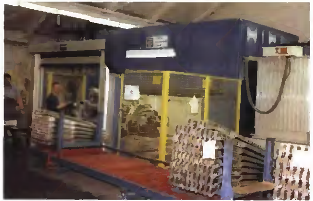
Fig. 7 — Project scheme and photograph of the round table NVEBW machine for structural beam production (1995).
