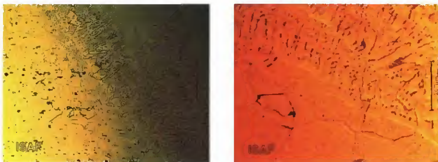
Fig. 11 — Nonvacuum electron beam welds on Al-0.4%Mg-1.2%Si transition zone to base metal, different magnifications.
