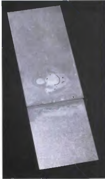
Coupons of Alloy 6111, 2 × 4 × 0.036 in. with 2-in. overlap. The top coupon has a 0.125-in. hole centered in the overlap area to facilitate introduction of Zn/15Al hard solder wire. Solder flows to every edge providing complete wetting of the joint.
