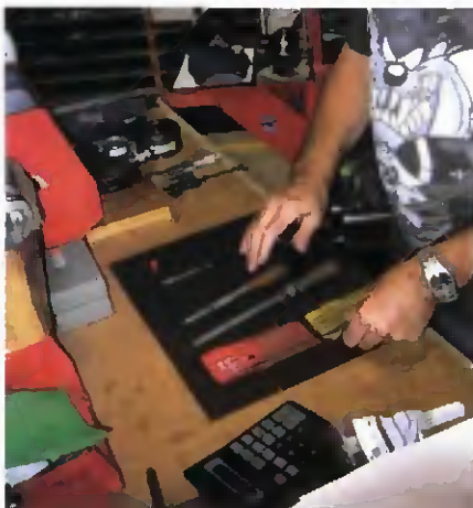
Fig. 8 — Jose Caldaron of Propulsion Technology Group likes to use these Nicholson files for final weld blending and deburring.
