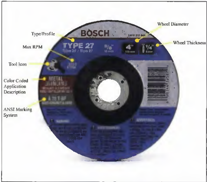
Fig. 4 — To make wheel selection easier, manufacturers burn a wide variety of information into the label, including a color-coded application description.
