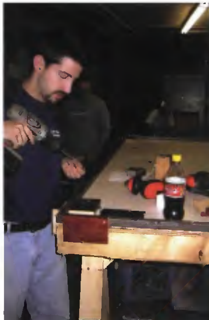
Fig. 10 — Prior to GMA welding of structures for theatrical sets, Phillip Blackwood uses his collection of Porter-Cable cordless drills to fasten holding blocks to this table.
