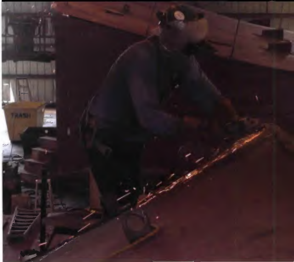
Fig. 5 — Proper eye protection and clothing should always be used whenever grinders are being used.
