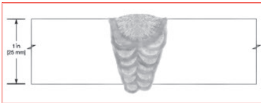
Fig. 1 — Cross section of multiple pass flux-electrode classification weld.
