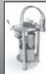
Guided Bend Testing Machine
