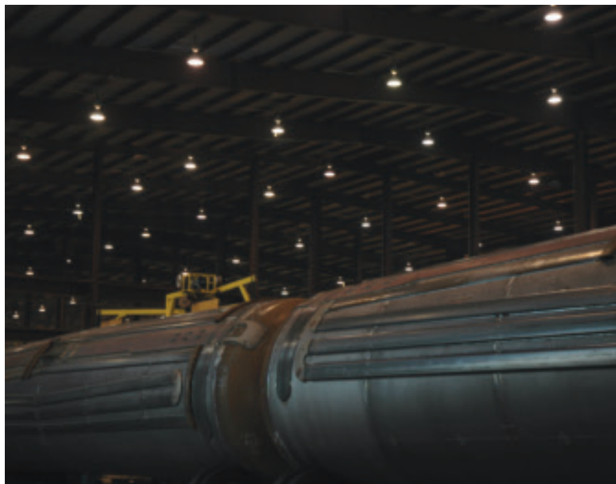
Fig. 7 — Hot water or steam will flow through the coils attached to this car to help liquefy the product it will carry.
