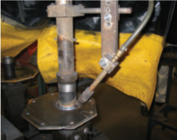
Fig. 1 — An example of hard automation where the welding gun is clamped in a fixed position.
