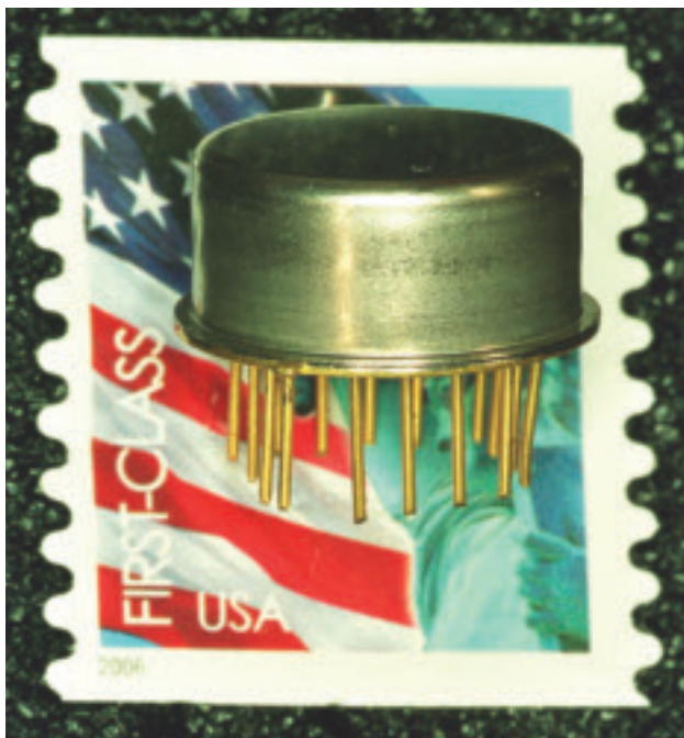
Fig. 2 — Vacuum-welded, 0.60-in.-diameter package.
