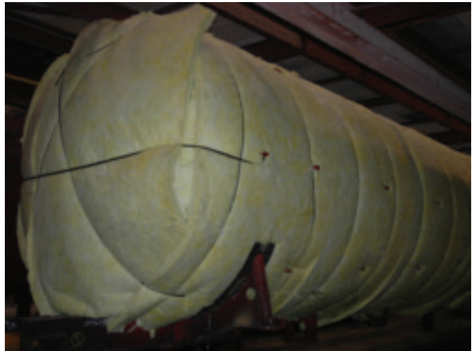
Fig. 11 — Jacketed cars receive a wrapping of insulation.
