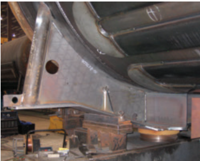
Fig. 5 — Bolsters such as these are welded to a bolster pad rather than to the tank itself.
