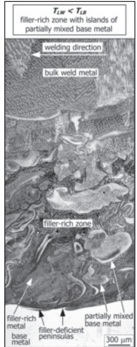
Fig. 5 — Longitudinal micrograph showing filler-rich zone with islands of partially mixed base metal in filler-rich metal and filler-deficient peninsulas along fusion boundary when T_{LW} < T_{LB} . Base metal: Ni; filler metal: Cu.
