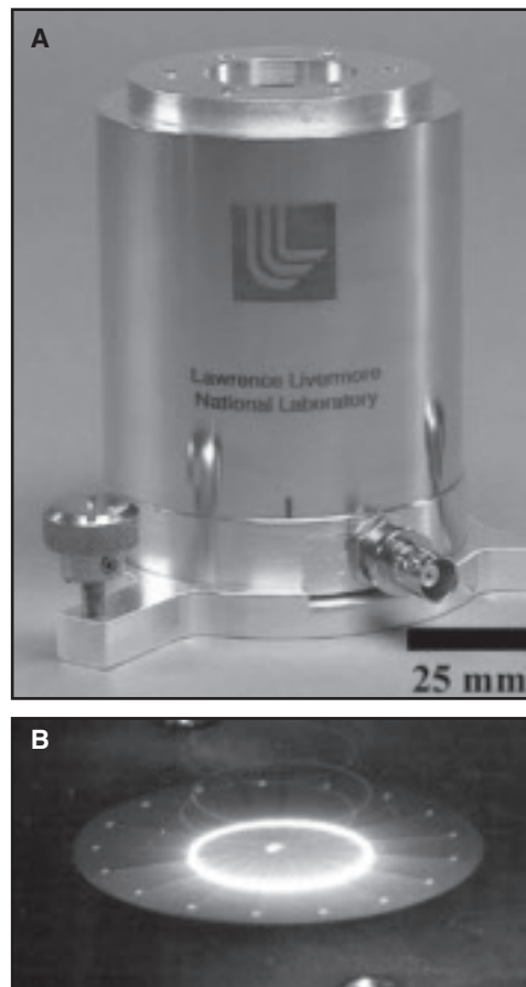
Fig. 1 — A — The Enhanced Modified Faraday Cup; B — an electron beam being deflected in a circular pattern over the radial slits in the tungsten slit disk located on the top of the EMFC.
