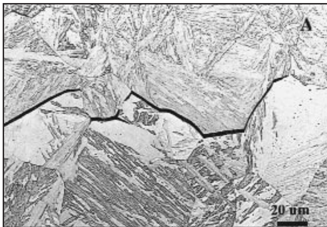
Fig. 2 — Representative LOM photomicrographs of failed samples viewed in cross section. Arrows indicate areas of void formation.
