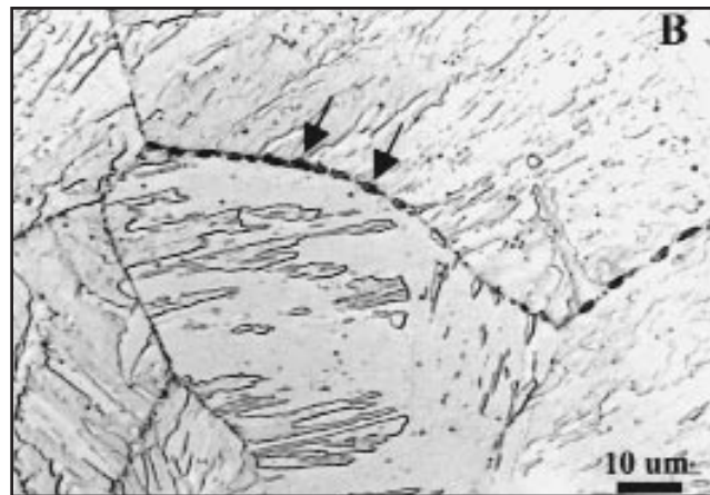
Fig. 2 — Representative LOM photomicrographs of failed samples viewed in cross section. Arrows indicate areas of void formation.
