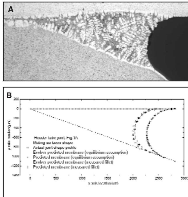
Fig. 9 — Header-tube brazed joint, side C, see Fig. 1A. A — Actual brazed joint. B — Comparison between an actual joint profile and the predicted topology. Comparison with Evolver calculations.
