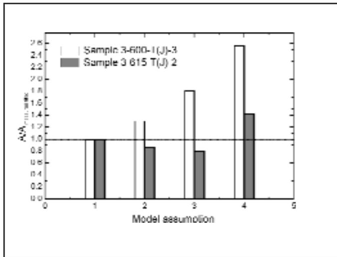
Fig. 12 — Comparisons of the predicted and measured fillet size areas ( $A = \text{fillet size}$ ): 1) measured fillet, 2) measured residue layer size, 3) nonequilibrium assumption, and 4) equilibrium assumption.
