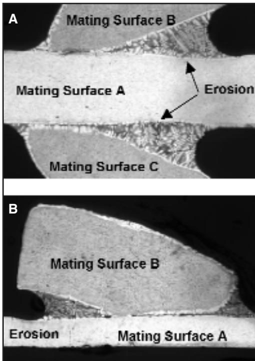
Fig. 1 — Cross-sectional views of a brazed joint. A — A configuration featuring multiple joints in a compact heat exchanger; B — a manifold extruded tube double-sided single joint. Detailed information about process conditions and materials is given in Ref. 3.
