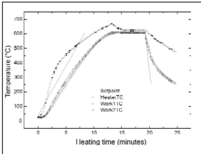
Fig. 3 — A typical ramp-up/dwell/quench temperature history of a CAB brazing process.
