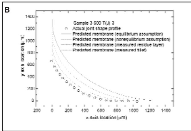
Fig. 5 — An inverted wedge-T joint. Brazing conducted at the peak brazing temperature of 600°C, dwell time 5 min. A — Actual brazed joint shape profile. B — Comparison between predicted and experiment data describing the joint topology. Predictions via 1) equilibrium phase diagram assumption, 2) nonequilibrium model of melting, 3) measurement of the residue, and 4) measurement of the fillet cross-section area.
