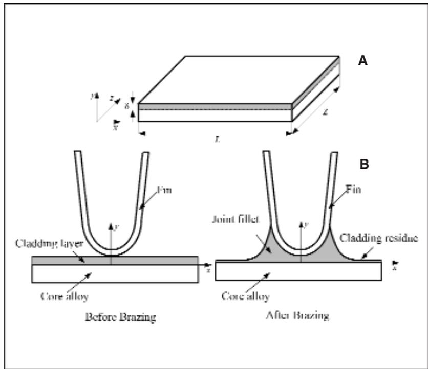
Fig. 2 — Schematics of: A — a brazing sheet ( $\delta = \delta_{clad}$  denotes cladding thickness and  $L$  and  $Z$  the 2-D length dimensions of the brazed joint corresponding sheet area); B — a compact heat exchanger fin-tube joint formation before and after brazing — a basic topology.
