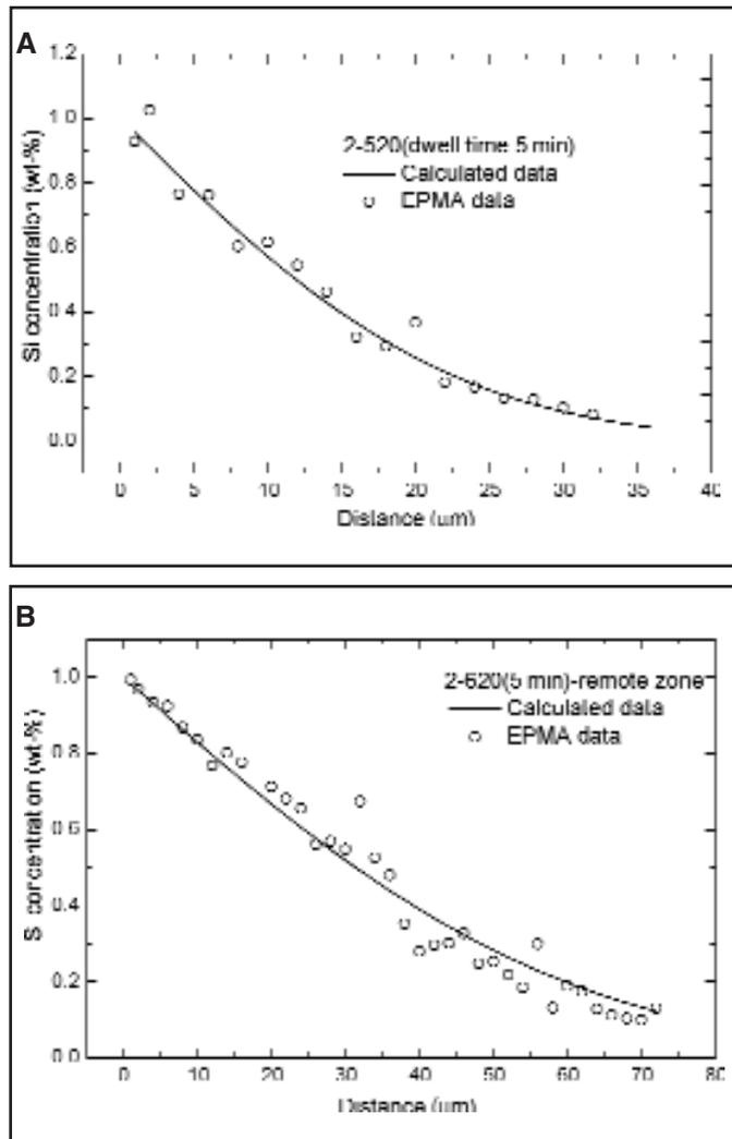
Fig. 4 — Silicon diffusion at the clad-substrate interface. A — No melting at 520°C, dwell time 5 min; B — a brazing process at 620°C, dwell time 5 min, residue location far from the joint zone. Alloys: core/clad AA3003/AA4343. For details of the diffusion patterns, see Ref. 1.
