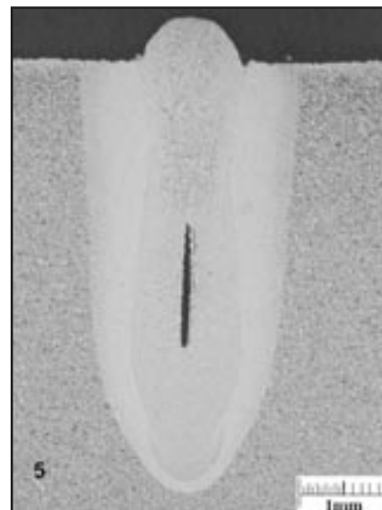
Fig. 11 — A typical centerline crack in laser welds (1045 steel, CO 2 laser, 6 kW, 2.5 m/min).
