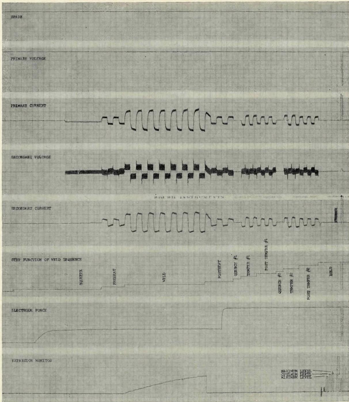
Fig. 1—Oscillographic traces of spotweld equipment parameters
