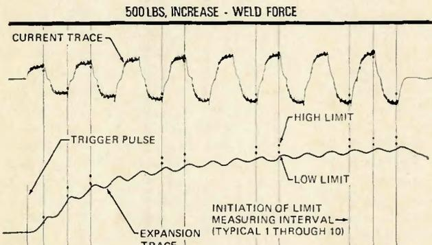
Fig. 8—Oscillograph recording of analyzer functions for a titanium spotweld detector; limits set for optimum weld—500 lb increase—weld force
