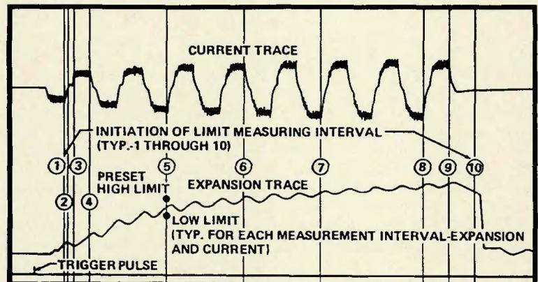
Fig. 3—Oscillograph recording of analyzer function for a conventional spotweld
