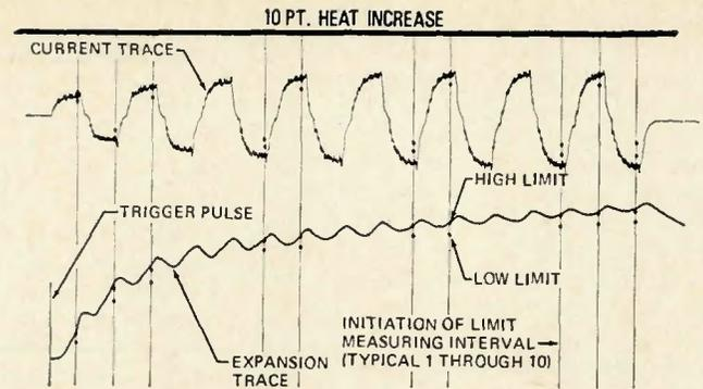
Fig. 5—Oscillograph recording of analyzer functions for a titanium spotweld; detector limits set for optimum weld—10 pt. heat increase
