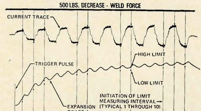
Fig. 9—Oscillograph recording of analyzer functions for a titanium spotweld detector; limits set for optimum weld—500 lb decrease—weld force
