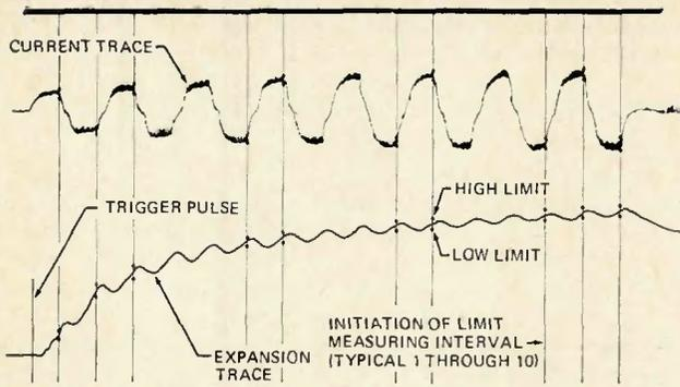
Fig. 4—Oscillograph recording of analyzer functions for a titanium spotweld detector limits set for optimum weld
