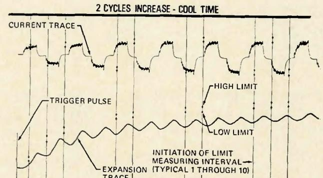
Fig. 7—Oscillograph recording of analyzer functions for a titanium spotweld detector; limits set for optimum weld—2 cycles increase—cool time
