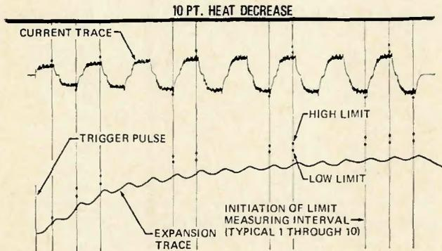
Fig. 6—Oscillograph recording of analyzer functions for a titanium spotweld; detector limits set for optimum weld—10 pt. heat increase
