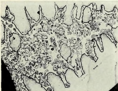
Fig. 6—Micrographic aspect of brazed joints obtained through the immersion process. Filler metal: 19 Cr-10 Si nickel-base alloy, oxalic acid etched. A (top) \times 8 ; B (center) \times 150 ; C (bottom) \times 300 (A reduced 54%, B and C reduced 50% on reproduction)
