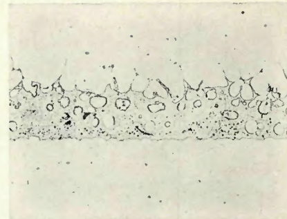
Fig. 3—Micrographic aspect of the stainless steel erosion by copper during brazing. Oxalic acid etch. \times 150 (reduced 50% on reproduction)
