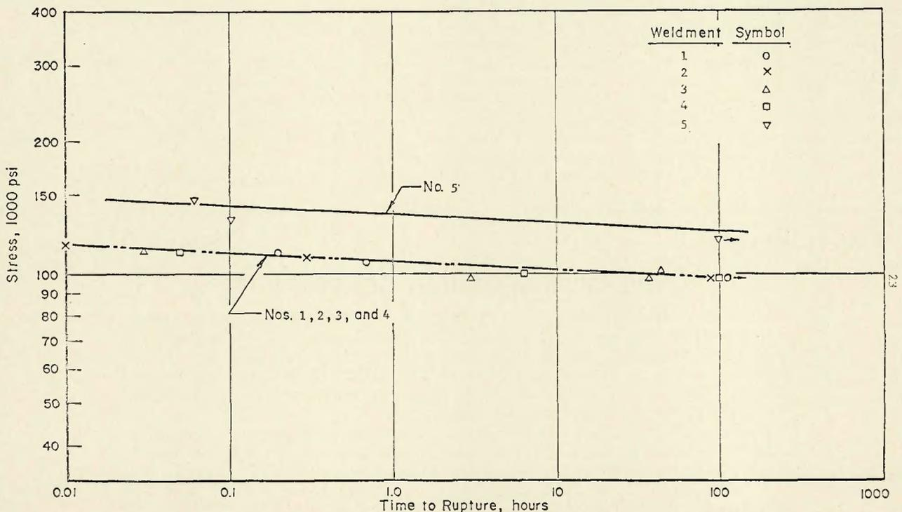
Fig. 4—Stress rupture curves for notched sheet samples at room temperature
