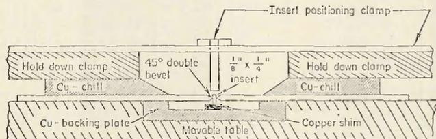
Fig. 1—Joint configuration and tooling for production of the weldments
