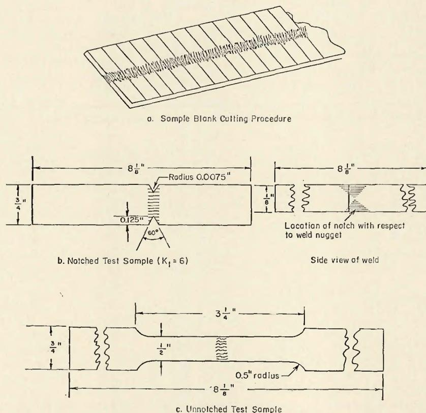
Fig. 2—Test sample location and sample dimension
