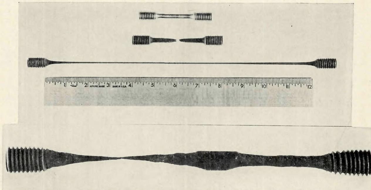
Fig. 6—Superplasticity is characterized by extensive neck free elongation. Top photograph shows machined tensile coupon, a broken non-superplastic coupon, and a coupon which exhibited superplasticity. A tensile coupon containing a weld at its center is shown in the lower photograph
