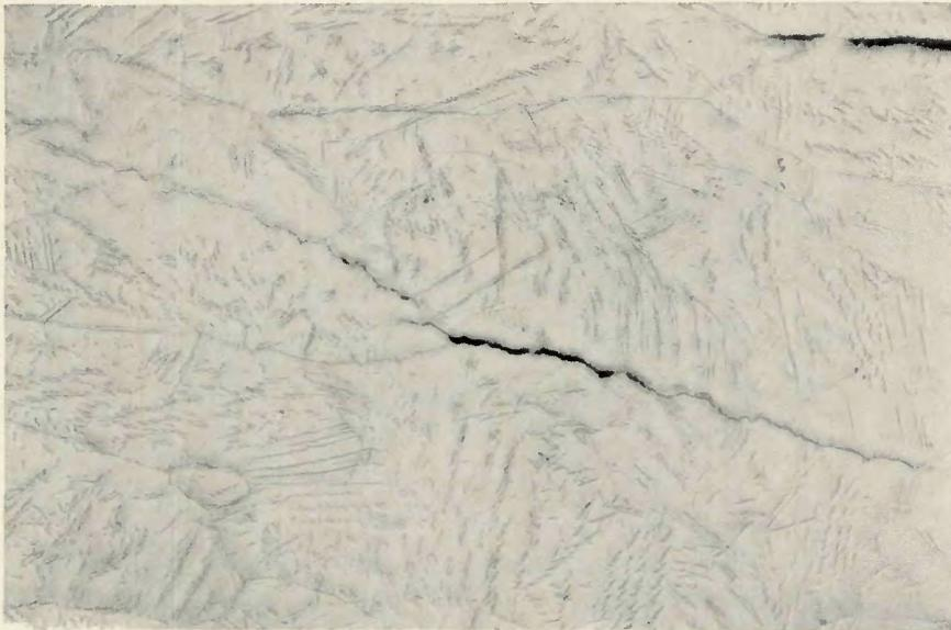
Fig. 1—Microstructure of gas metal-arc weld made with a commercial Type 312 stainless steel filler metal. The matrix is ferritic with austenite precipitated randomly and at grain boundaries. Weld solidification cracks were intergranular. Etchant: electrolytic 10% oxalic acid, X100 (reduced 22% on reproduction)
