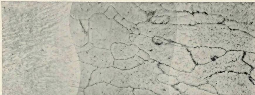
Fig. 5—Composite picture showing the base, heat-affected zone, and weld deposit in a gas metal-arc weld in IN-744. Etchant: electrolytic 10% oxalic acid. X75 (reduced 55% on reproduction)
