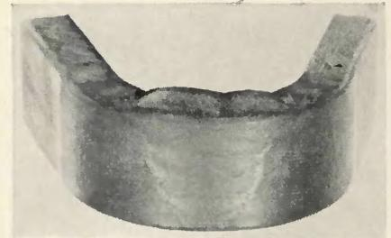
Fig. 2—Weld soundness under severe conditions is shown by this defect-free transverse slice from a 1 in. thick gas metal-arc weld after bending 180 deg
