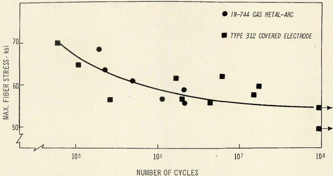
Fig. 3—R. R. Moore fatigue test results on smooth bars containing welds at centers made with filler metals and processes shown
