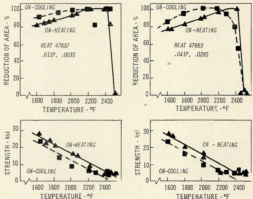
Fig. 4—Hot ductility behavior of two heats of IN-744 containing low and high levels of phosphorus and sulfur
