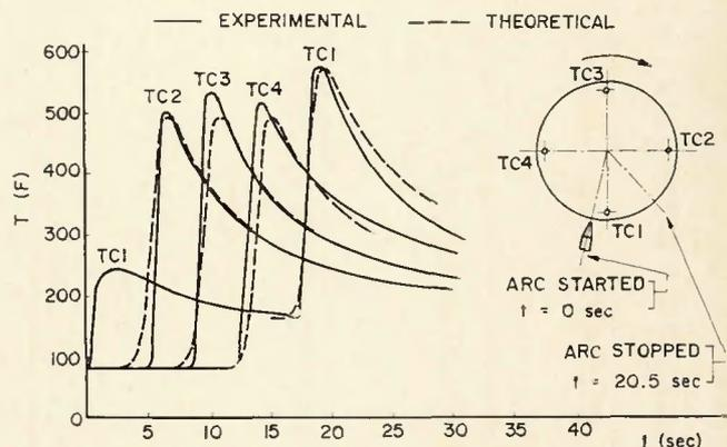
Fig. 4—Comparison of theory and experiment for circumferentially grouped thermocouple locations
