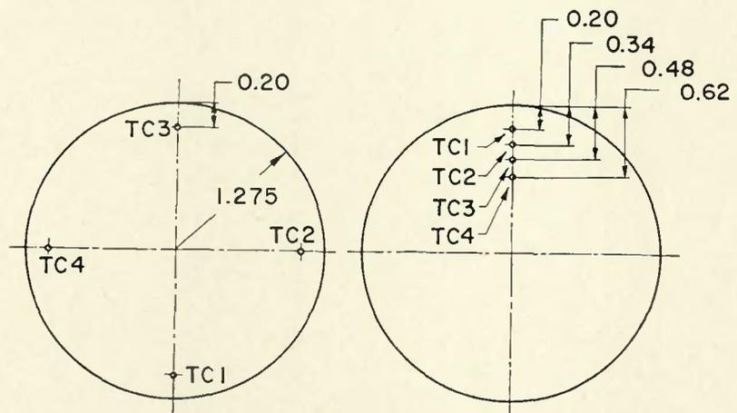
Fig. 2—Location of circumferentially and radially grouped thermocouples
