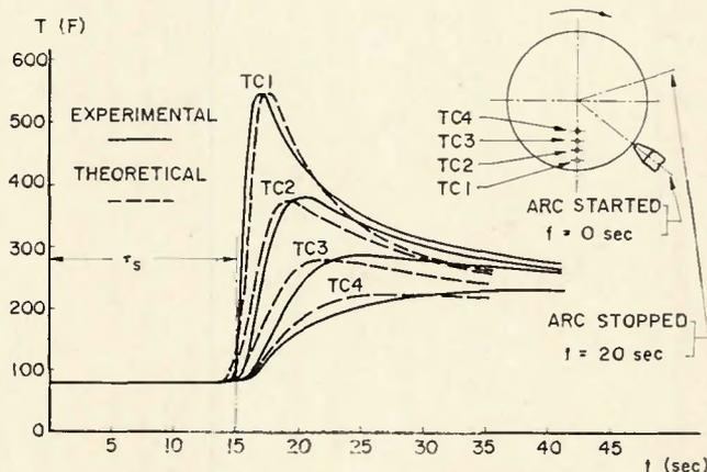
Fig. 3—Comparison of theory and experiment for radially grouped thermocouple locations
