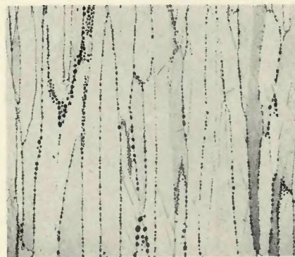
Fig. 2—CVD tungsten after high-temperature anneal. Etched with H_2O_2-NH_4OH . X100 (reduced 50% on reproduction)
